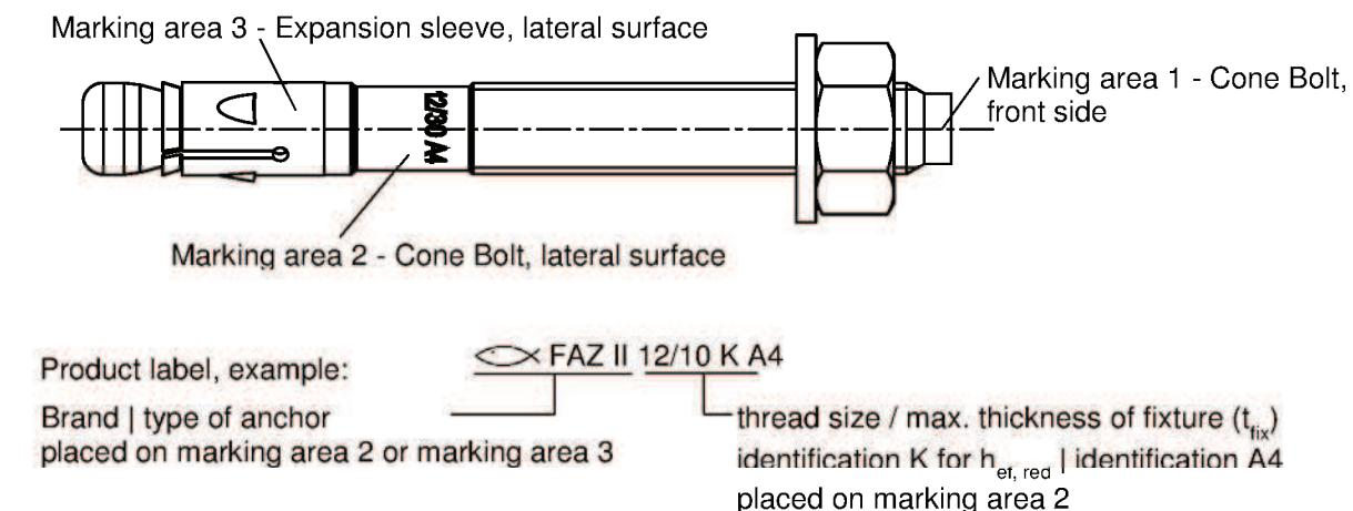
**Table A2:** Letter-code on marking area 1 and maximum thickness of fixture  $t_{fix}$ :
