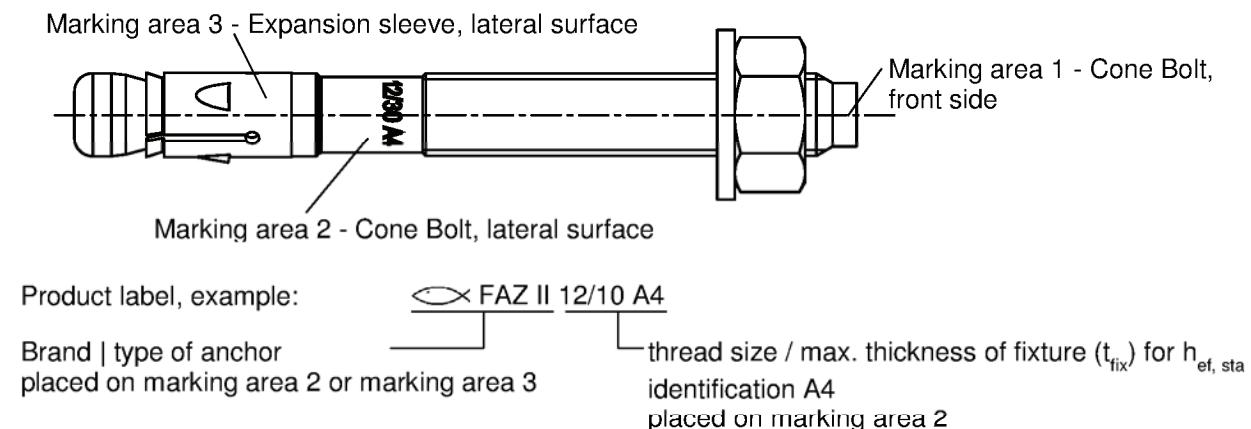
**Table A1:** Letter-code on marking area 1 and maximum thickness of fixture  $t_{fix}$ :
